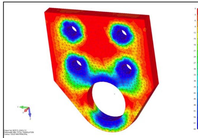
This detail shows the minimum principal strains for a metal bracket with bolt preload and contact surfaces.
